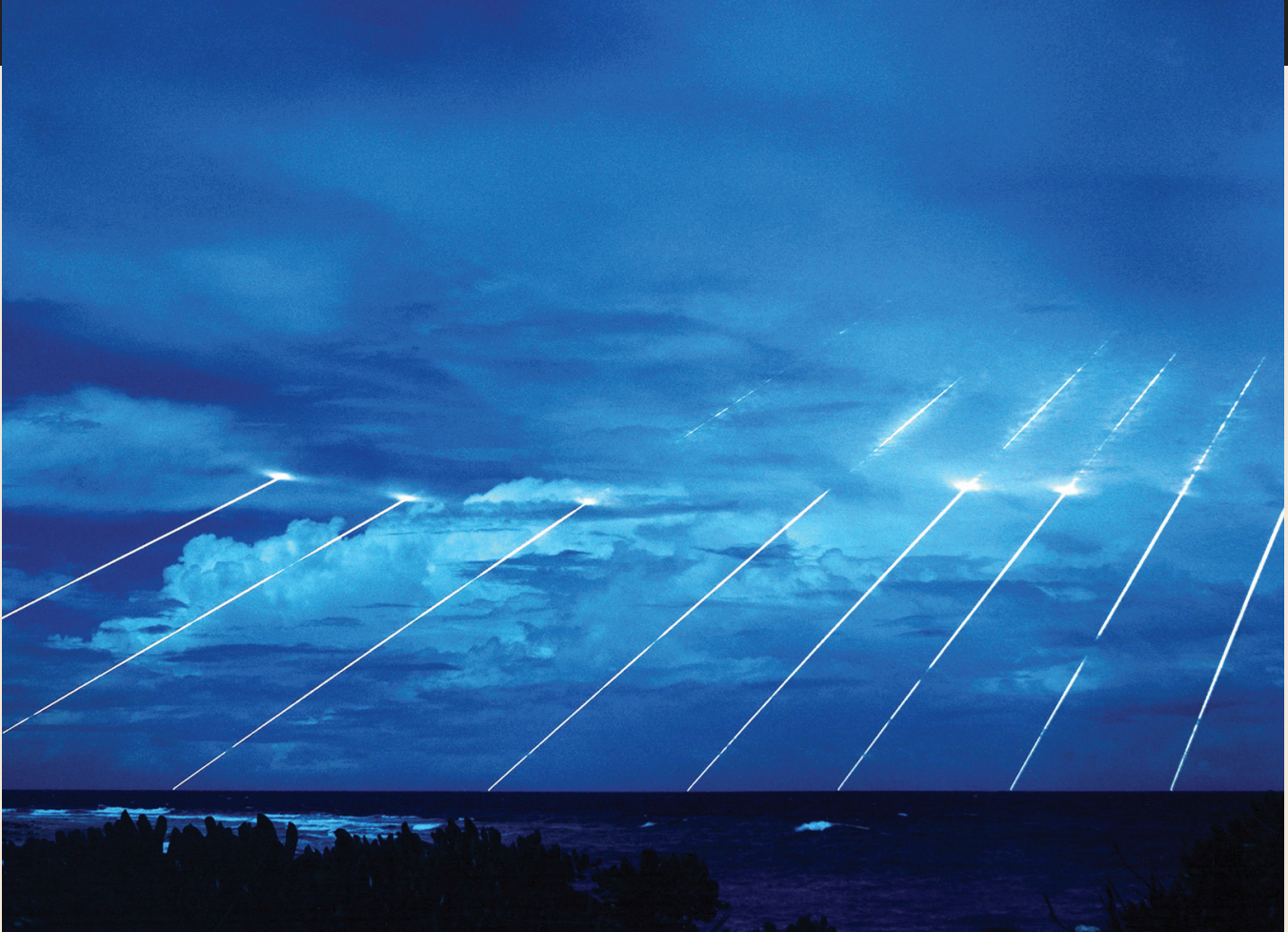
A Peacekeeper test missile re-entering the atmosphere at the Kwajalein Atoll in the Marshall Islands. This long exposure photo shows the paths of the multiple re-entry vehicles deployed by the missile. Each of the missile's 10 nuclear warheads could be aimed to destroy a different target and packed a yield that was many times greater than Fat Man or Little Boy. (Photo: U.S. Army.)
